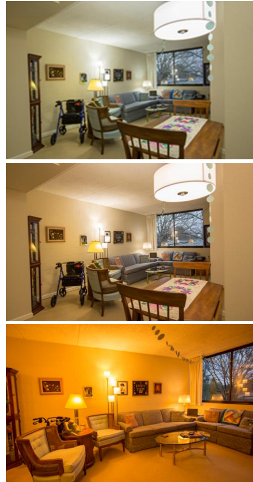
Figure 10: During waking hours, the Stack lamps were programmed to automatically change kelvin temperatures from 5000K to 2200K as shown above.
