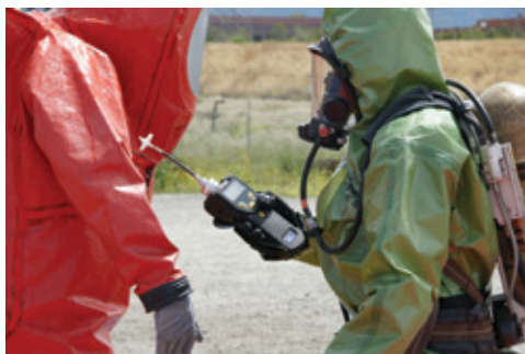
FIGURE 4.3.6. PID for decontamination monitoring
